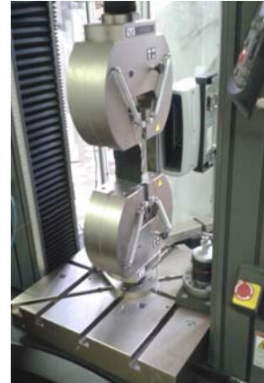
Figure 2 Textile reinforced composite with integrated textile sensors during electromechanical measurement
