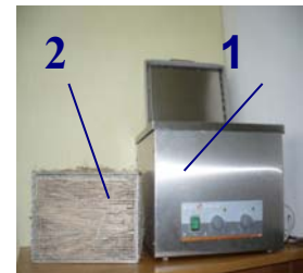
Fig. 2 Washing device Sonic 14 (1) and (2) container with the straw
