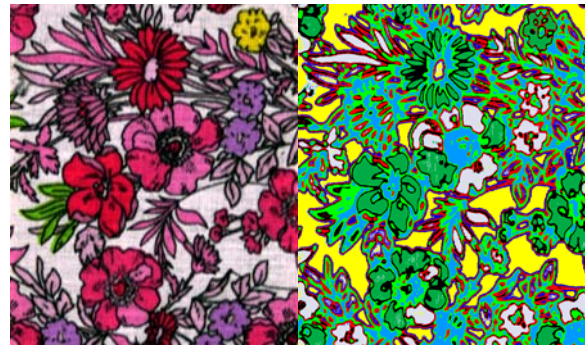
Figure 6 Printed fabric sample and segmented color regions
