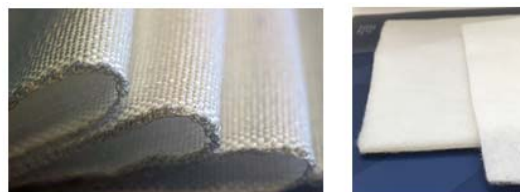
Figure 1 Fabric and nonwoven obtained with new PLA based fibres
