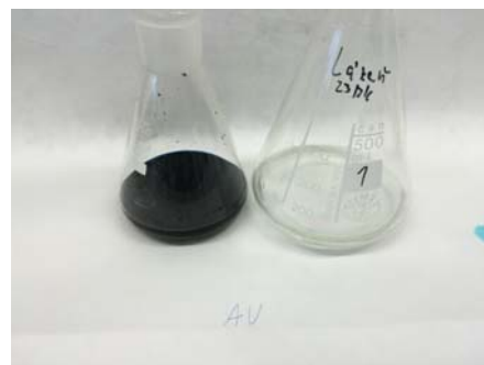
Figure 1 Picture of spent black dyeing bath and the same bath treated by precipitation and subsequent adsorption .
