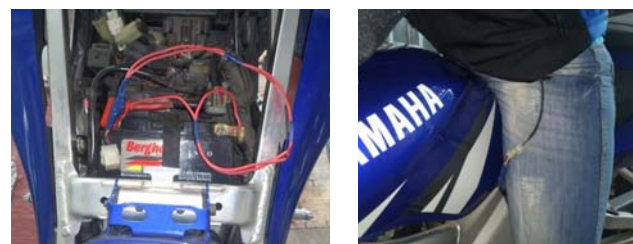
Figure 2 Connection of the heating element to the motorcycle
