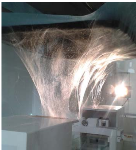
Figure 1 Needleless electrospinning of a PAN solution with undesired cotton-candy-like polymer connections between high voltage electrode and substrate
