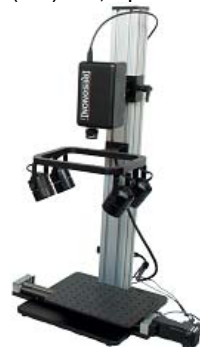
Figure 2 Hyperspectral imaging camera (PIKA L, Resonon Inc., Bozeman, USA)
