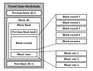
Figure 2. The TrustChain blockchain architecture
