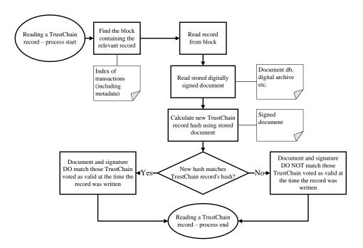
Diagram 3. Reading a record from the TrustChain
