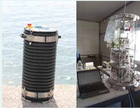
The first SEA-on-a-CHIP prototype with the outer casing on (left) and off (right). The second prototype will be smaller, more energy efficient and more efficient in its use of chemicals.
