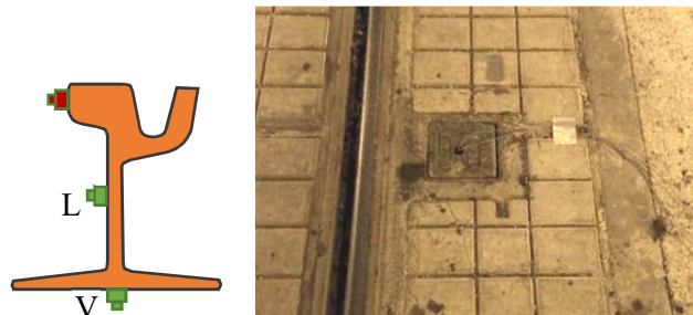
Figure 6. Position of accelerometers on a rail foot (vertical direction) and rail web (horizontal direction), inside a small shaft.
