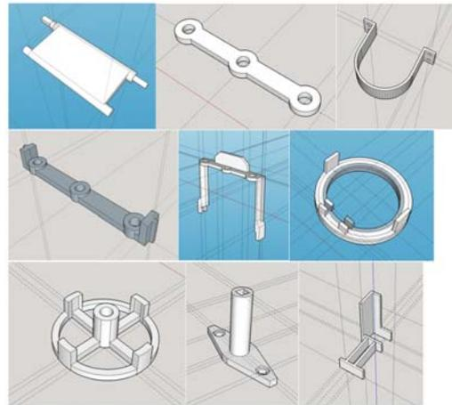
Fig. 4. Example of 3D designs of printed mechanical parts of the catamaran.
