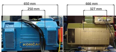
Fig. 4: Comparison of induction machine (left) and IPM machine (right)
