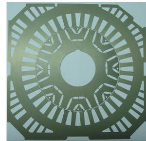
Fig. 3: Stator and rotor laminations of the IPM motor
