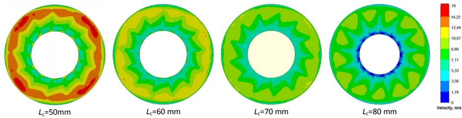
Fig. 9: Influence of router length  $L_c$  on the fan inlet flow/velocity distribution
