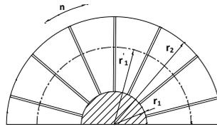
Fig. 7: Radial blade centrifugal fan (radial cross section)
