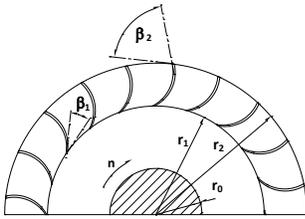
Fig. 6: Backward curved blade centrifugal fan (radial cross section)
