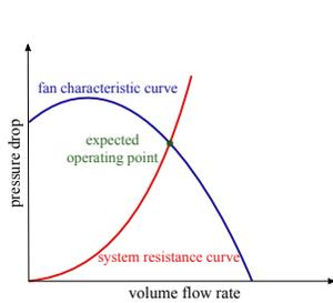
Fig. 1: Centrifugal fan and system resistance curves
