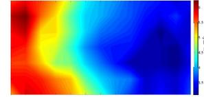
Fig. 12: Measured air velocity profile across the outlet surface
