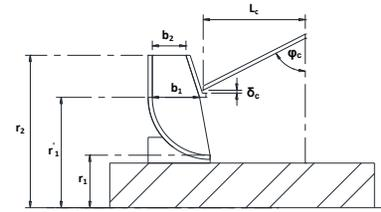
Fig. 8: Radial blade centrifugal fan (axial cross section)
