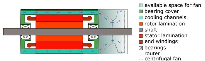
Fig. 5: Machine cross section
