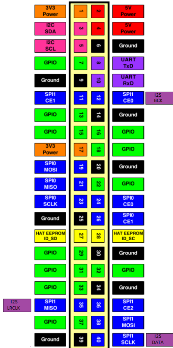
Slika 2.2 Raspored GPIO pinova
