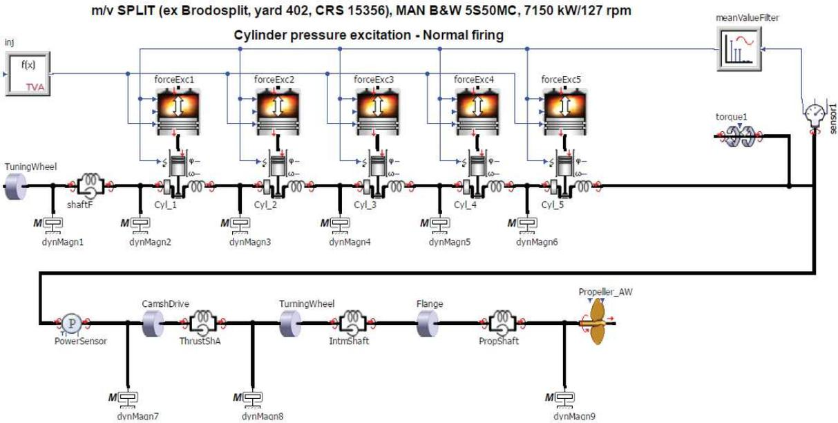
**Figure 2** SimulationX shafting model for the calculation of torsional vibrations
