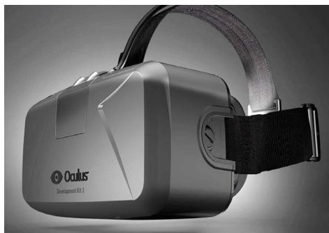
Fig. 2. The Oculus Rift head-mounted display for dynamic stereoscopic viewing
