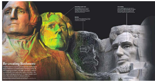
Fig. 10. A composite image produced by the National Geographic Magazine of the digital recording of the Mount Rushmore heads
