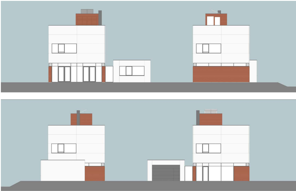
Fig. 7. Four facades of the AA10 project, generated on the basis of a 3D model Source: Jack Breen, The AA Variations Project.
