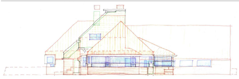
Fig. 5. Combination of two, overlaid, explorative analytical hand-sketches on transparent paper, simultaneously showing the front and side facade of the AA4 project
