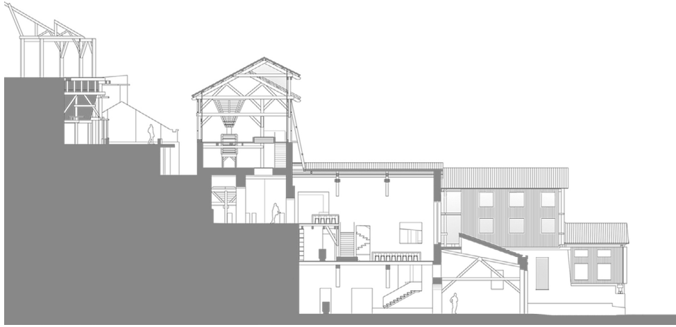
Fig. 3. Cross-section of the Washery at Argentiera, Sassari (Italy)
