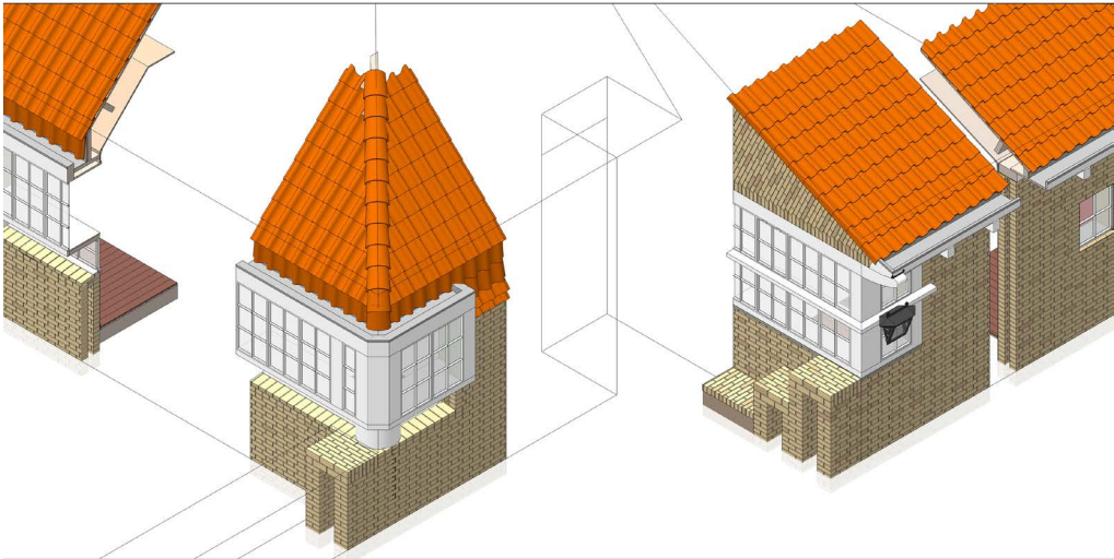
Fig. 6. Combination of sectional 3D models, showing critical details and features of the AA4 project's expressive front and side facades
