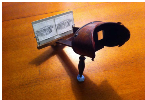
Fig. 1. An early stereoscopic viewing device with computer-generated wire-line stereo pairs of a building
