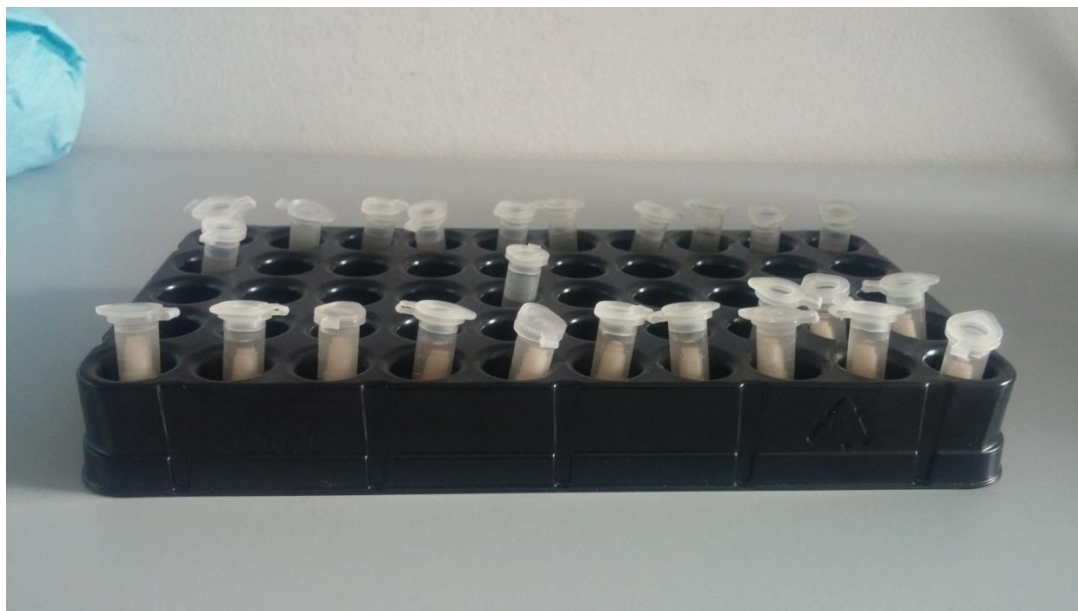
Figure 7. Implants placed in Eppendorf tubes containing bacterial suspension. Implants covered in their entire length by the bacterial suspension
