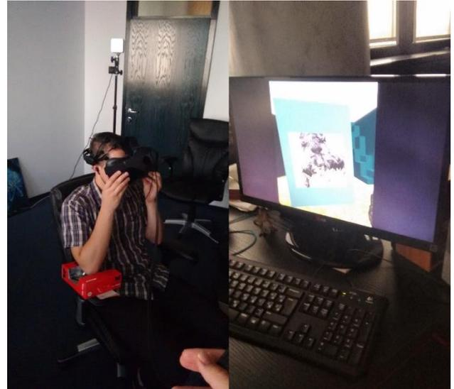
Fig. 6. On the left, a participant is wearing VR and EEG headsets during the experiment. One of the HTC Vive VR sensors is visible in the background. The supervisor station is on the right.
