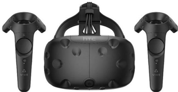
Fig. 1. HTC Vive headset (center) and controllers (left and right) [21].
