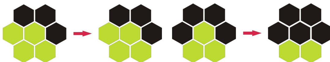
Figure 3. Two characteristic examples of center cell adaptation to its surrounding by the majority rule, left: without change, right: with a change of state.
