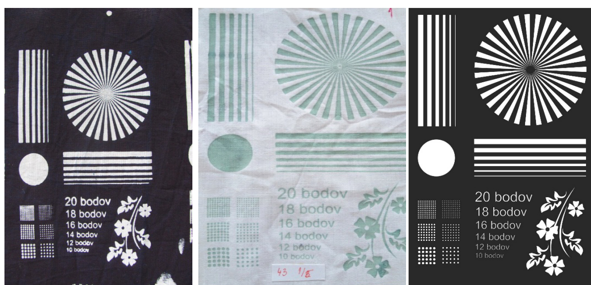
Figure 1. Design of the print pattern (left), reserve printed on the cotton fabric (middle), finished sample after printing, dyeing and washing (right).
