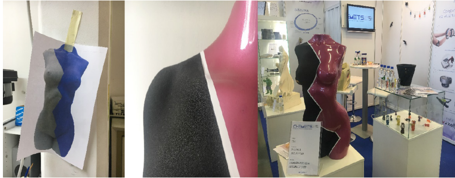
Figure 5. Sand printed natural sized torso.
