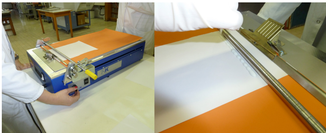
Figure 1. Application of the barrier coating on the RK Multicoater K303.
