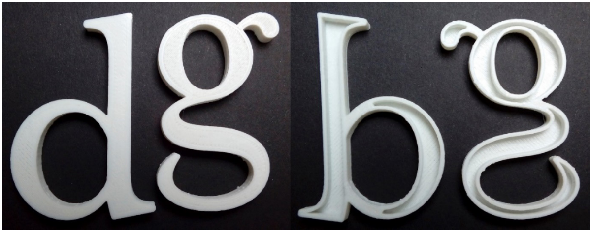
Figure 2. Letters "d" and "g" with corrected errors of uncompleted surfaces.
