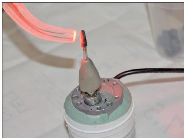
**Fig 1** The implant placed on the rotational electric motor and treated with the light source (LAD), 5 mm away from the implant.
