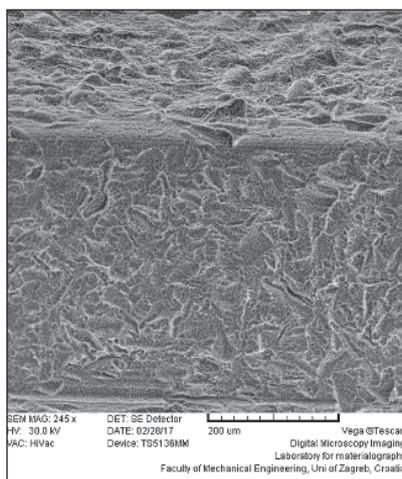
**Fig 5** (Right) Implant treated with LAD; magnification 1:250.
