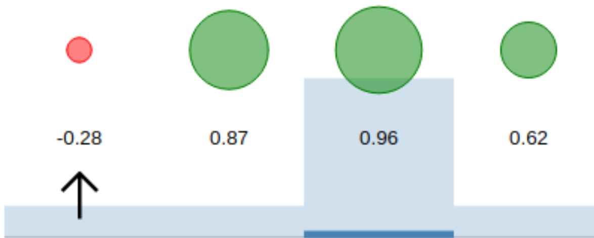
Figure 12: Probability distribution based on the epsilon-greedy algorithm where the action with the largest Q value has a probability of being selected 1 - \epsilon , whereas the rest are evenly distributed.
