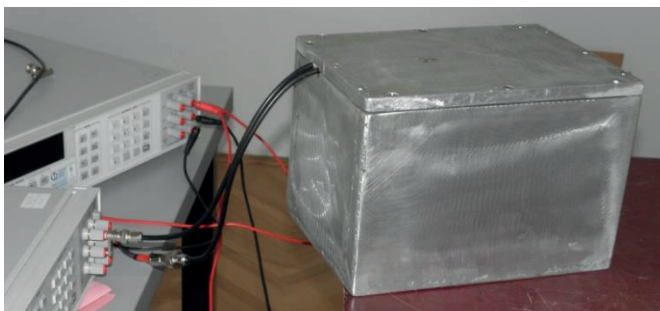
Figure 11. Assembled time constant standard during resistance measurement
