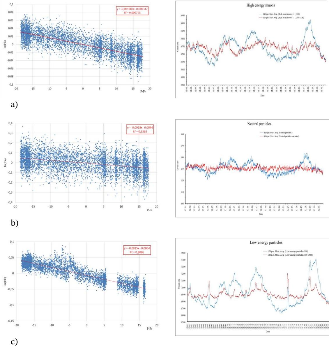
Fig. 2 Graphs for barometric coefficient are on the left side, from top to bottom; a) high energy muons, b) neural particles and c) lower energy particles (with excluded data, see Tab. 1.). On the right side are the monthly smoothed graphs with moving average which show corrected data using the barometric coefficient.
