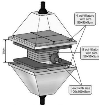
Fig. 1 SEVAN particle detector module schematic. The corresponding signals: 100 – traversal of the low energy charged particle. 010 – traversal of the neutral particles, 111, 101 – traversal of the high energy muons ( $> 250$  MeV). SEVAN CRO is located on latitude 45.82 N; longitude 15.97 E; altitude 170 m; vertical cut-off rigidity  $\approx 4.9$  GV
