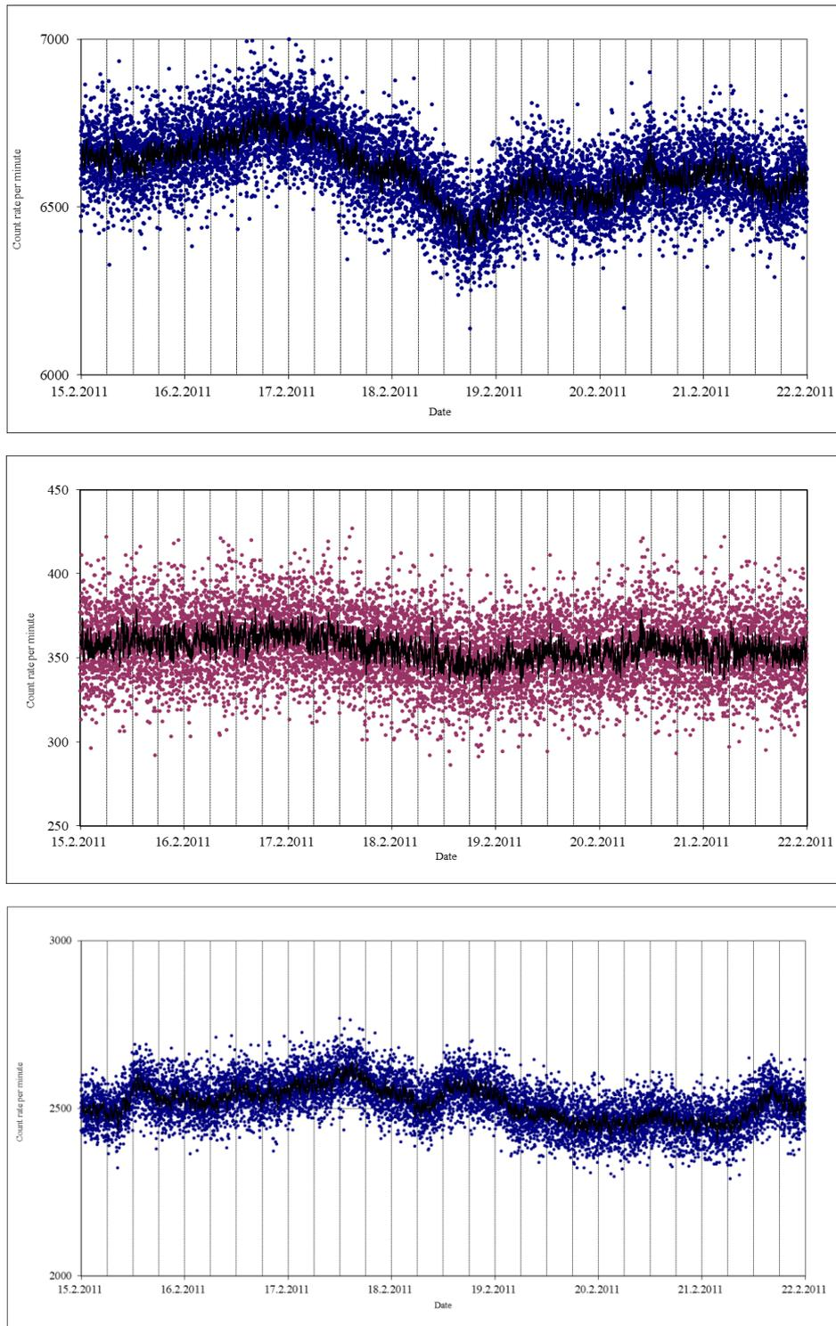
*Fig. 3 Forbush decrease detected on SEVAN CRO instrument showing from top to bottom: low energy particles, neutral particles, high energy muons*
