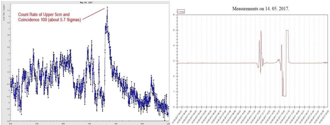
Fig. 5 On the right side is the measurement of disturbance in electric field, the measurements are relative and the instrument is not calibrated during the lightning event. On the left side is the TGE enhancement in upper 5cm plastic scintillator and coincidence of “100” (mostly low energy electrons and gamma rays) where we can see an increase in count rate during a lightning.
