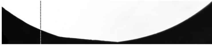
Fig. 1. (111) facet and its neighbourhood projected directly on photographic paper (rotated 90° counter-clockwise, magnification  $52.51 \pm 0.03$  times, digitised with 2540 dpi, 255 grey levels, image size  $5499 \times 26710$  pixels). The resolution obtained is  $0.1904 \pm 0.0001 \mu\text{m}$ . The row of pixels analysed in Fig. 2 is indicated by dashed line.
