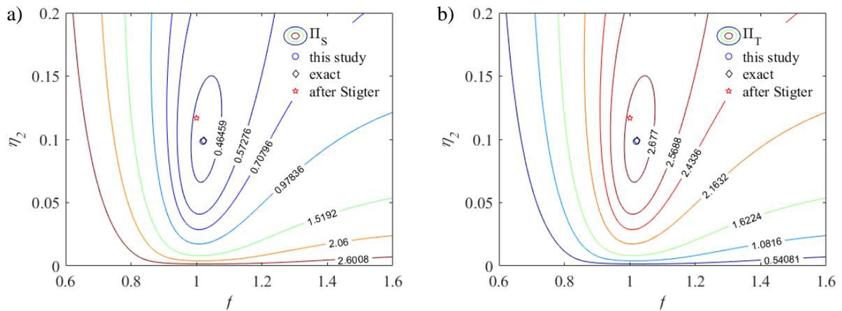
Figure 4: a) The dimensionless absorbed power index of the tank and b) the dimensionless index of the power dissipated by the ship, as functions of the frequency ratio and the ART damping ratio with  $\mu_1 = 0.0046$ , and  $\eta_1 = 0.0075$
