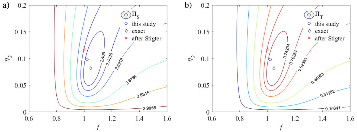
Figure 3: a) The dimensionless absorbed power index of the tank and b) the dimensionless index of the power dissipated by the ship, as functions of the frequency ratio and the ART damping ratio with  $\mu_1 = 0.046$ , and  $\eta_1 = 0.075$
