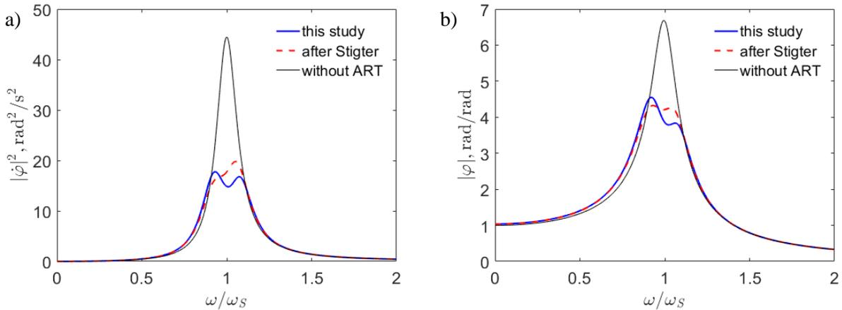
Figure 2: a) the roll velocity squared b) the roll angle as a function of frequency per unit excitation wave angle
