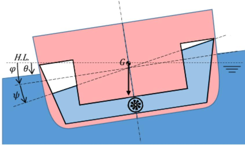
Figure 1: The scheme of a ship equipped with an anti-roll tank
