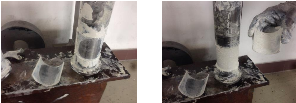
Figure 4: Steel pin before (left) and after the (right) lubrication
