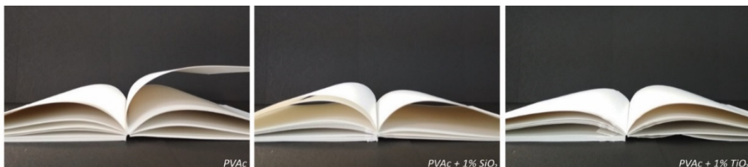
Figure 3: Opening behaviour of CW book blocks (PVAc; PVAc + 1%SiO 2 ; PVAc + 1%TiO 2 )
