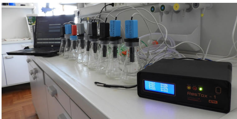
Figure 1: ResTox, a respiratory activity measuring system comprising multiple sensors based on NDIR technology.
