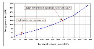
Fig. 4. Steam turbine energy power loss change during the developed power variation for operating point 1
