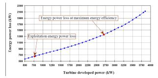
Fig. 6. Steam turbine energy power loss change during the developed power variation for operating point 3
