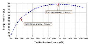
*Fig. 7.* Steam turbine energy efficiency change during the developed power variation for operating point 5
