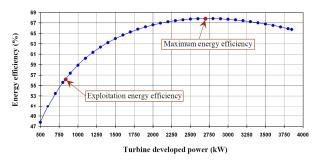
Fig. 3. Steam turbine energy efficiency change during the developed power variation for operating point 1
