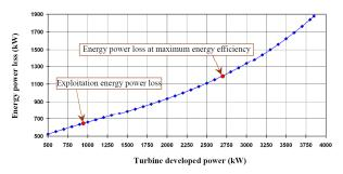
*Fig. 8.* Steam turbine energy power loss change during the developed power variation for operating point 5
