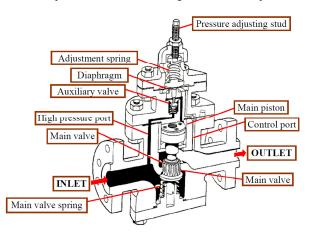
Fig. 1. Analyzed steam pressure reduction valve intersection [9]
