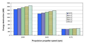
Fig. 6. Change in the exergy destruction of analyzed valve during the ambient temperature change
