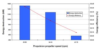
Fig. 5. Exergy destruction and exergy efficiency of the pressure reduction valve - exploitation
