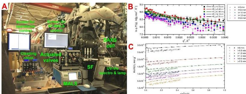
A-The SF-MALS-SAXS set up in the SWING beamline hutch; B, C, a selection of SAXS (B) and MALS (C) processed data at 0.5 min intervals derived from a fibrin monomer (0.16 mg/mL) re-polymerization experiment.
