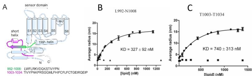
Figure 1. A) Schematic representation of the TRPA1 receptor showing the regions predicted to interact with lipids and those investigated herein. B and C) Interaction of the peptides with POPC (♦) and POPC/PIP<sub>2</sub> (●) by MDS.
