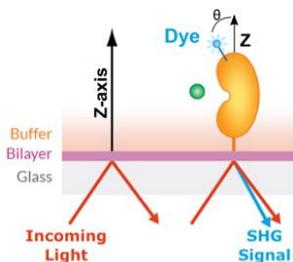
*SHG signal intensity depends on physical orientation of the dye. Small discriminatory changes in dye orientation are captured by SHG signal change*
