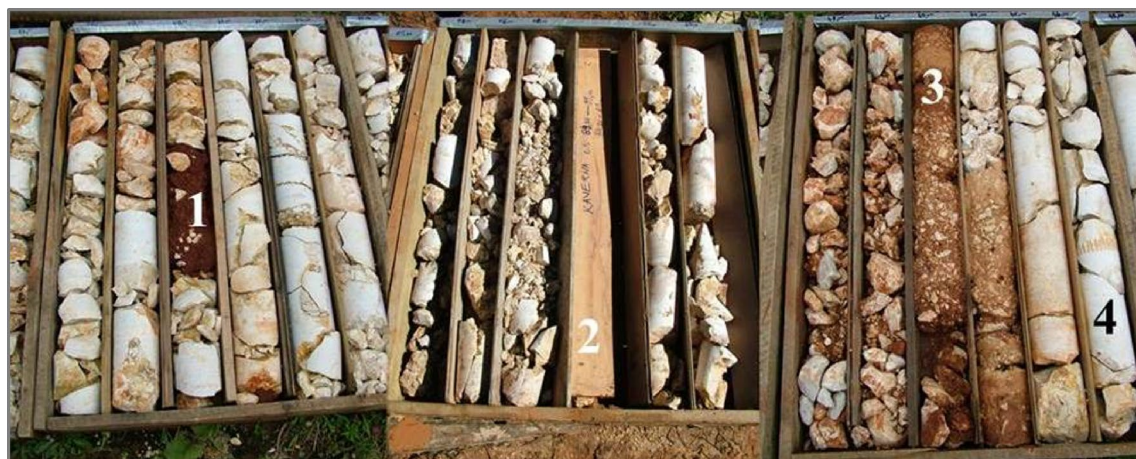
Fig. 2 Different materials in the rock mass of Zadar borehole: (1) terra rossa ; (2) cavern; (3) rock fragments and terra rossa —partially solidified; (4) fractured rock
