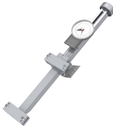
Figure 5. Innovative, lateral force measuring device
