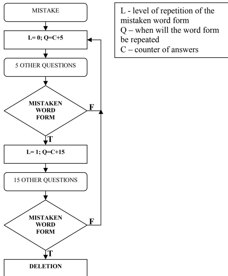
Picture 2 – Graphical representation of the algorithm for mistakes handling in CALCOR 0.3
