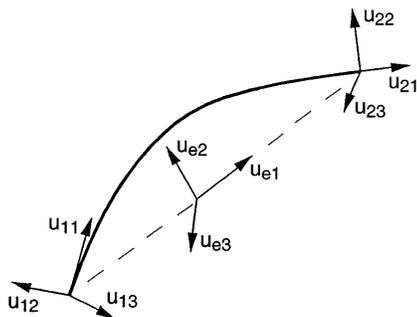
Fig. 2. Two noded deformed beam element
