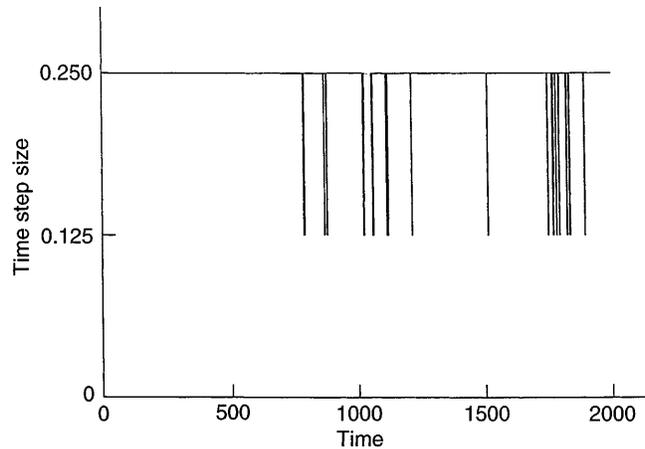
Fig. 5. Example 1, time step halving for the mid-point algorithm
