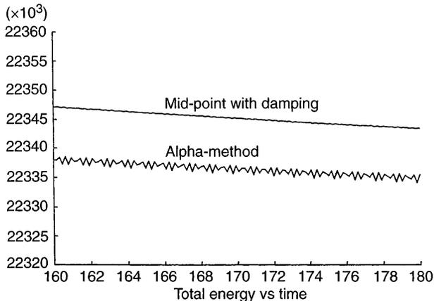
Fig. 8. Example 2, differences in the damping characteristics between the mid-point scheme and the  $\alpha$ -method
