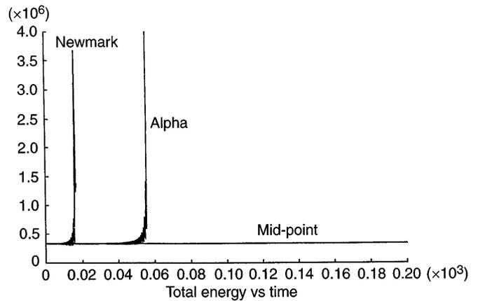
Fig. 10. Example 3, total energy vs time for Newmark,  $\alpha$  and mid-point (with no damping) schemes
