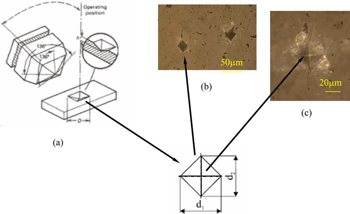
Figure 1. Vickers hardness testing. a) Schematic of a Vickers or diamond pyramid hardness indenter. The indentation depth  $h$  is approximately  $1/7$  of the average length  $D$  of the diagonals [4]. b) Vickers indentations on a radial cross section of 99.8 %  $\text{Al}_2\text{O}_3$  ceramics. The load on the indenter was  $1 \cdot 9.81$  N (HV1), and the dwell time was
