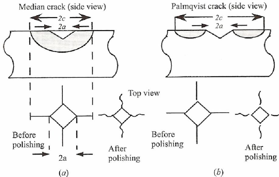
Figure 2. Crack system developed from the Vickers indents. (a) Side and top views of a median crack, (b) top and side views of a Palmqvist crack [2].
