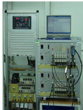
**Fig. 3.** The assembled test system consisting of a VCU and a PC on top of it.
