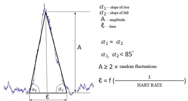
Fig 2. Decision parameters for burst identification
