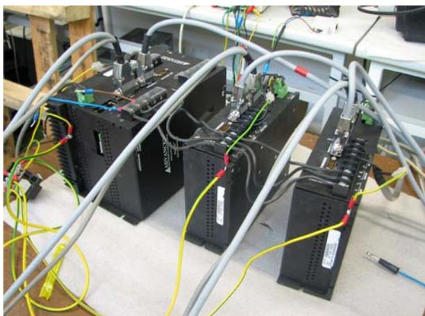
Figure 5. Servo controllers
