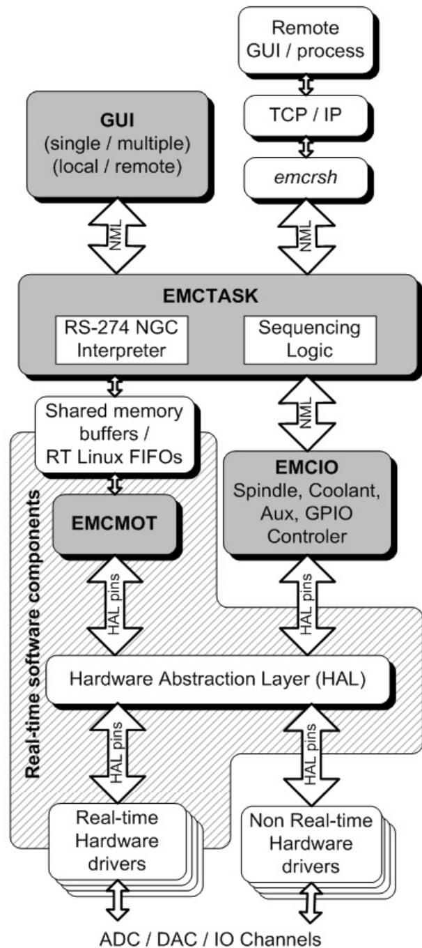
Figure 1. EMC Architecture
