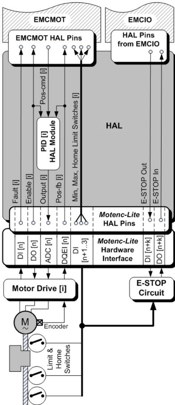
Figure 3. HAL configuration for testbed
