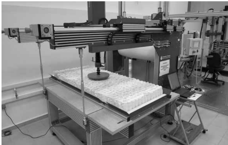
Figure 8. Device for determining mattress durability and elasticity
