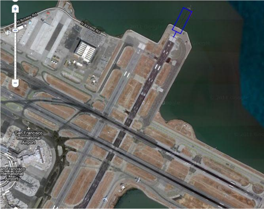
Figure 2 RESA according to Annex 14 at the threshold 19 at San Francisco Airport
