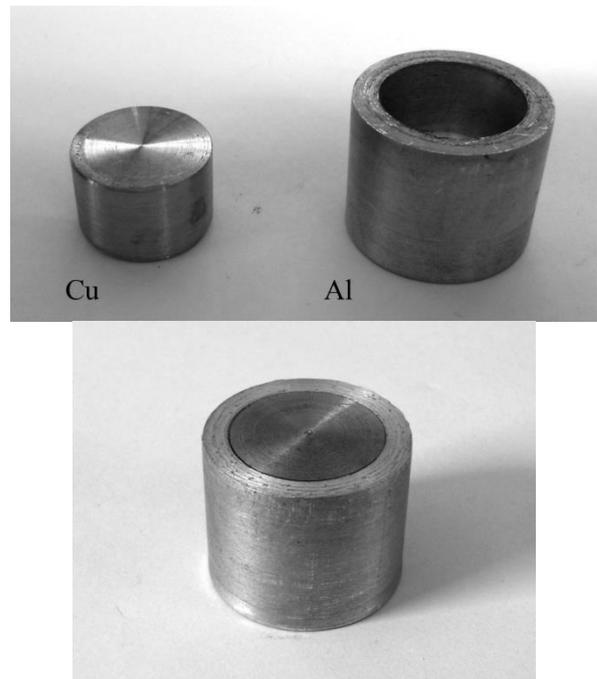
Fig 3. Photograph of separated copper and aluminium parts
