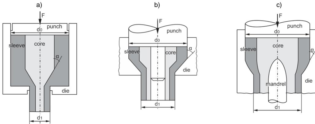
Fig. 1 Different variants of bi-metallic extrusion a.) forward extrusion b. and c.) tube extrusion
