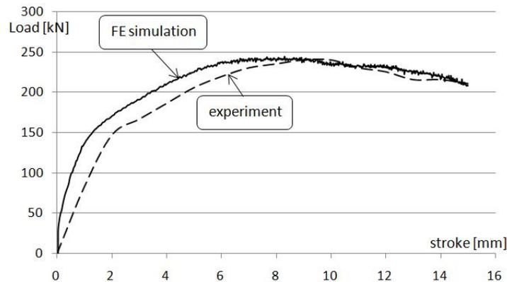
Fig. 7. Load stroke diagrams obtained by experimental investigation and FE simulation
