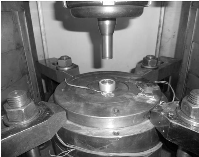
Fig. 4. Tooling for bi-metallic backward extrusion
