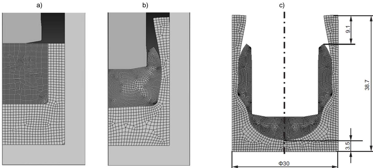
Fig. 6. Numerical simulation: a) start, b) intermediate phase after 6 mm punch stroke and c) end of the process (full cross-section)
