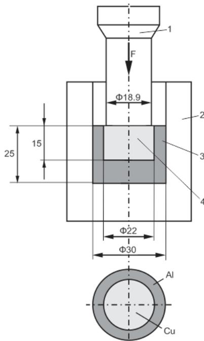
Fig. 2. Configuration of billet and die
