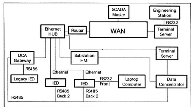
Figure 1: Typical integrated substation protection and control system [8]
