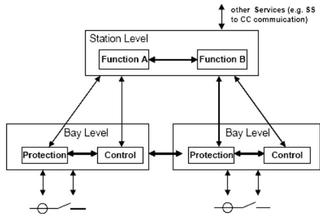
Figure 2: Typical substation automation system
