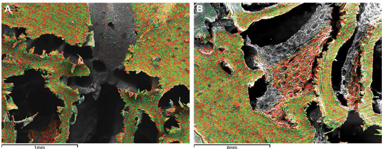
**FIG. 3.** Mapping of the chemical elements on the Er:YAG laser-irradiated site (A), and bur drilling site (B).
