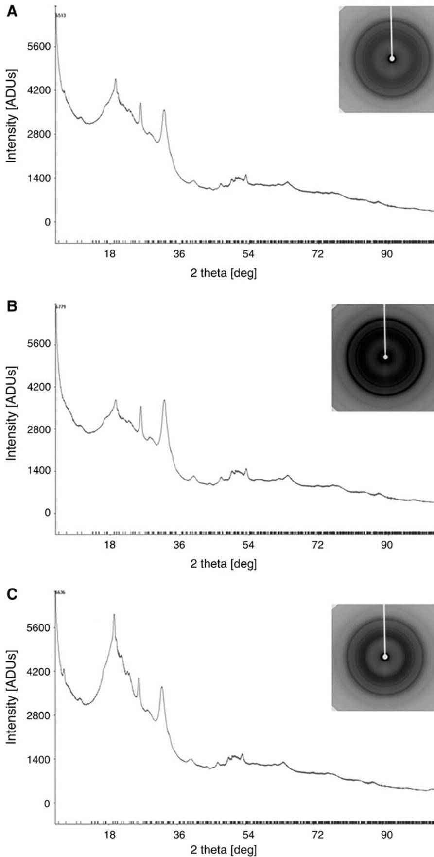
**FIG. 5.** Diffractograms and diffraction images of x-ray diffraction (XRD) analysis. **(A)** Er:YAG laser irradiation (1000 mJ/pulse, 20 Hz) under saline solution irrigation. **(B)** Cortical bone site after bur drilling. **(C)** Untreated bone tissue and pure hydroxyapatite.
