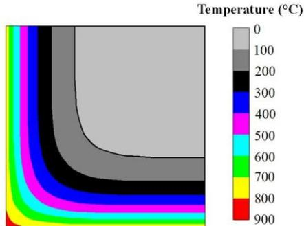
Figure 4. Temperature field in one quarter of a column after 30 minutes of ISO fire [4].
