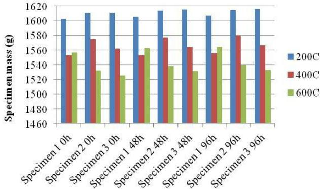
Figure 3. Mass change of specimens from mix3 during 96 hours after cooling.
