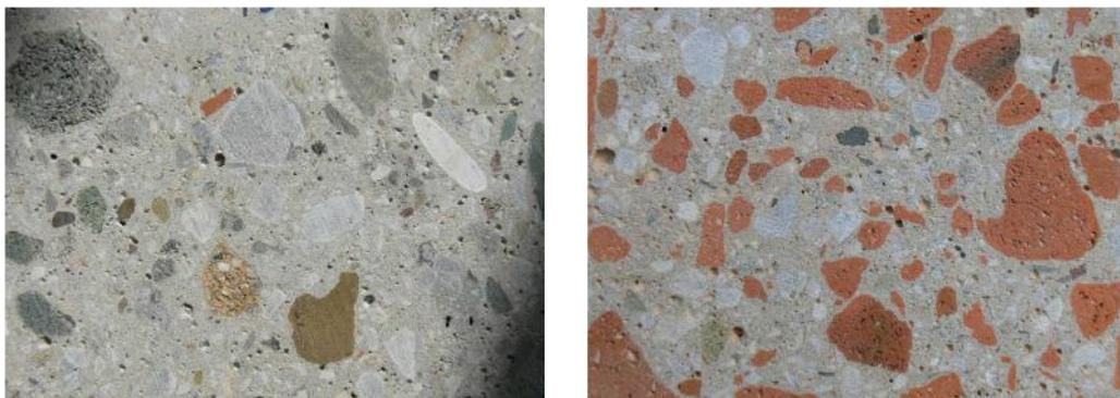
Figure 1: Surface of the specimen with recycled concrete aggregates (left); and with recycled brick aggregates (right)
