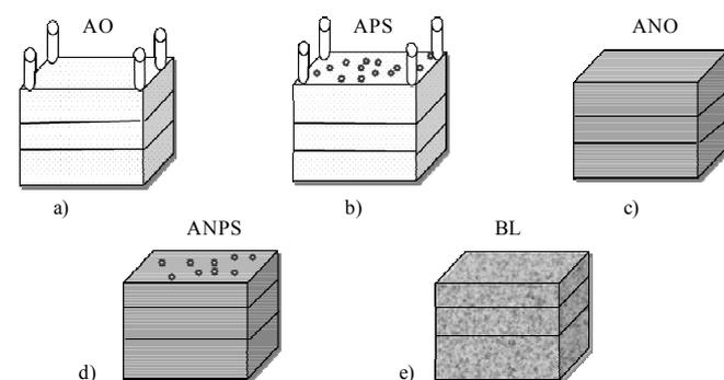
**Figure 1.** Design of composting piles: a) AO – aerobic conditions without bacterium, b) APS – aerobic conditions with bacterium, c) ANO – anoxic conditions without bacterium, d) ANPS – anoxic conditions with bacterium, e) BL – spontaneous degradation without bacterium and forced aerating.
