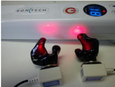
Fig 1: Individual ear plugs with embedded optical cable
