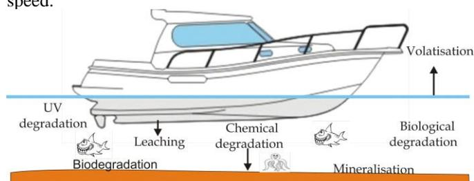
FIG 1. EFFECT OF ANTI-FOULING LEACHING
