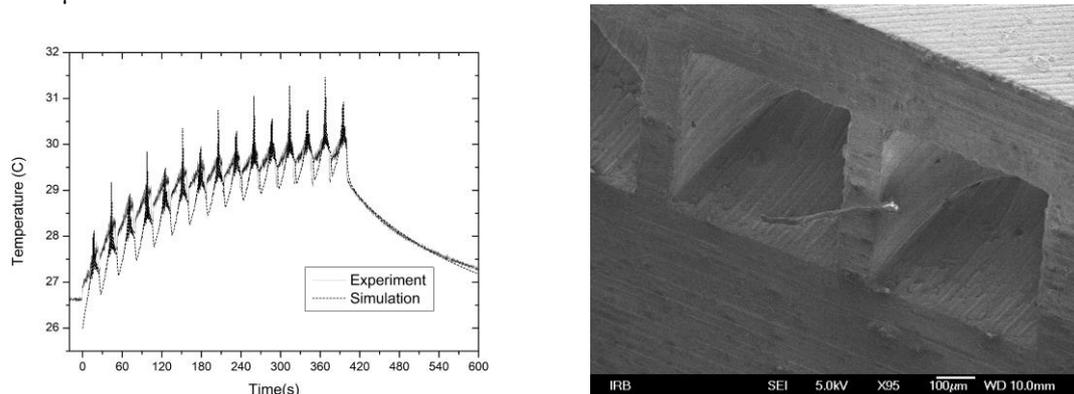
Fig. 2. Measured temperatures during fs laser operation with numerical simulation, left panel. SEM image of dental cavities formed by fs laser, right panel
